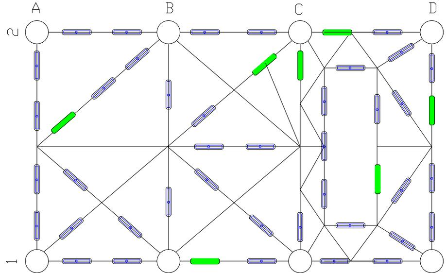
Anodes oriented ≈ “East-West”... such as the one on the D1 HZ → D2 , are designated as (oriented) E-W. Measurements on these are taken with the diver (and clip) on the ‘ *southernmost* ’ side of the anode (leftmost side of drawing).
